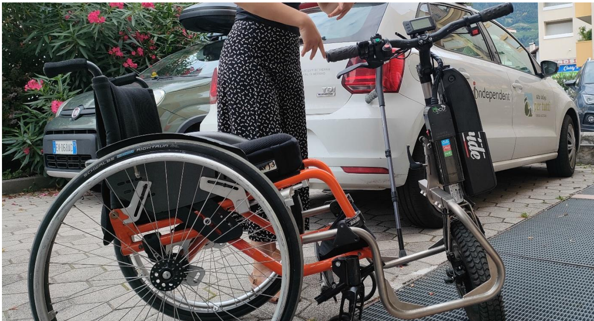
Figure 2 Example of an accessible traction device for people with disabilities
